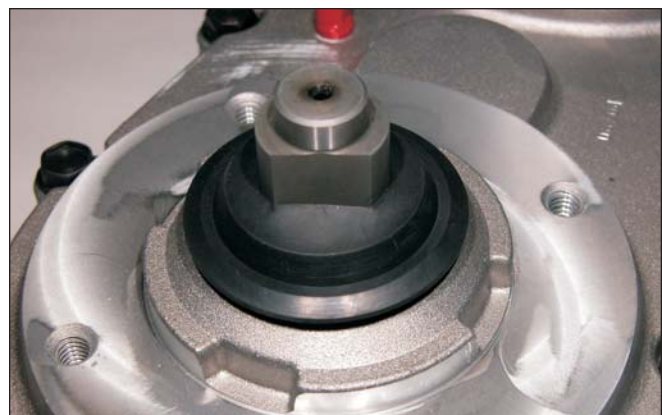
Output shaft with water shed
