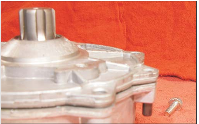
Place cover on gear box. Drive in alignment pins before inserting & tightening screws.
