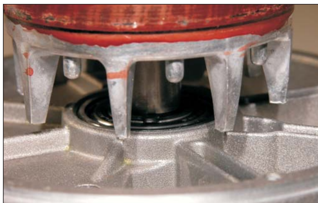
Rotor bearing seated properly
