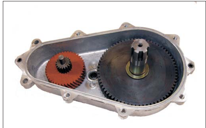
First gear and output gear installed
