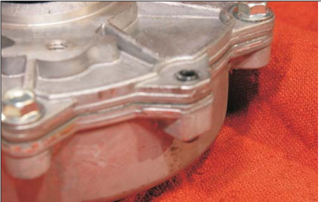
Check assembly, be sure alignment pins are in and bolts tight.
