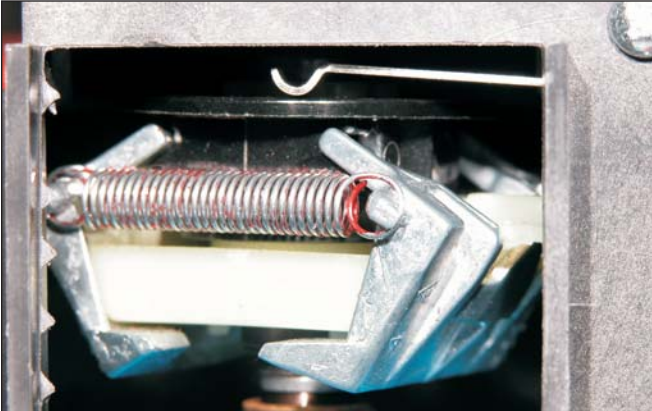
At rest, switch must be open
