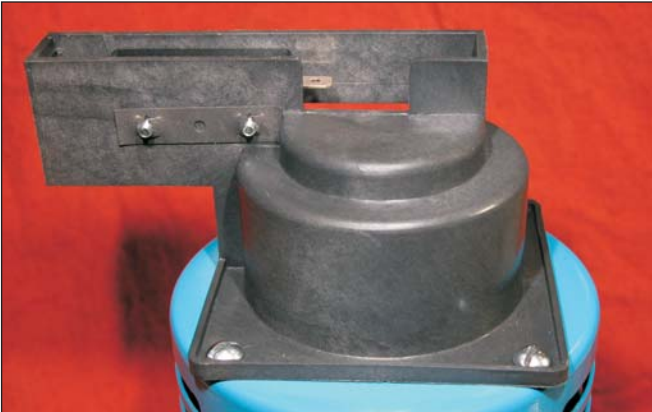
Add switch cover, secure motor & cover to gear reducer
