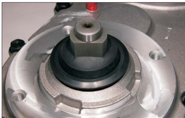
Output Shaft and Water Shed
