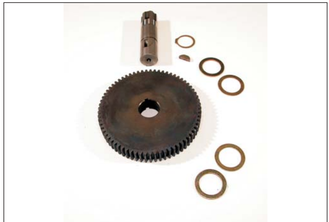
Prior Output Gear, Shaft, Key, Snap Ring, Washers and Spacers
